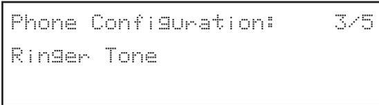
2. The current ring tone is displayed. Use the ↑ and ↓ keys to access the desired ring tone. As you scroll through the selections, the ring tone can be heard for three seconds. When the desired ring tone is displayed, press **Select**.
